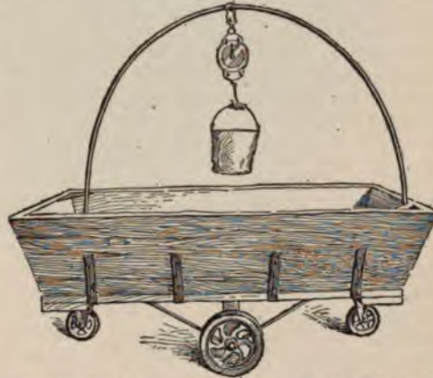
Fig. 342. Truck and scales used in weighing grain feeds.
